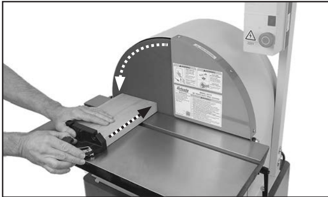
Figure 10. Example of Y-axis sanding.
